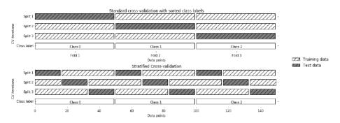
Figure 5-2. Comparison of standard cross-validation and stratified cross-validation when the data is ordered by class label
