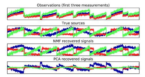
Figure 3-19. Recovering mixed sources using NMF and PCA
