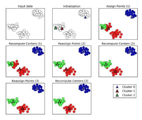
Figure 3-23. Input data and three steps of the k-means algorithm
