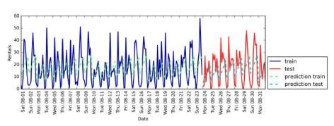
Figure 4-16. Predictions made by linear regression using day of week and hour of day as features
