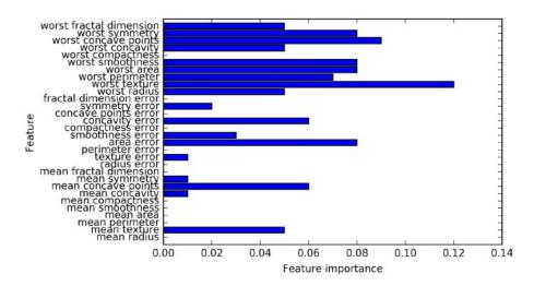
Figure 2-35. Feature importances computed from a gradient boosting classifier that was fit to the Breast Cancer dataset
