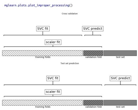
Figure 6-1. Data usage when preprocessing outside the cross-validation loop
