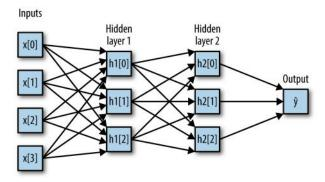
Figure 2-47. A multilayer perceptron with two hidden layers
