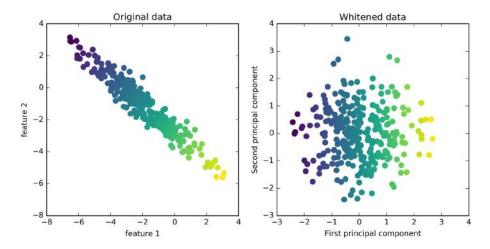
Figure 3-8. Transformation of data with PCA using whitening
